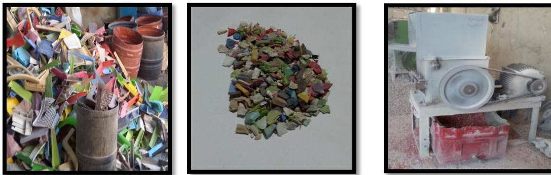
Fig. (1a): Plastic Waste Fig. (1b): Crushed Plastic Waste Fig. (1c): Crusher of Plastic to Pieces of about 12 mm Waste
